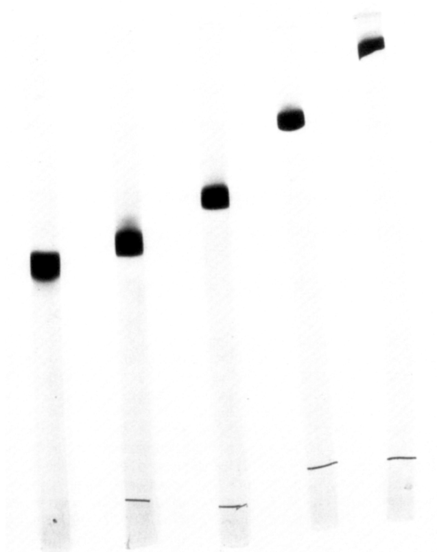
Fig. 1 Polyacrylamide gel electrophoretogram of 9.5 \mu g H. eutropha RuBP carboxylase. The electrophoresis was done on gels polymerized from (left to right) 4, 5, 5.5, 6.5 and 7.5% acrylamide.
